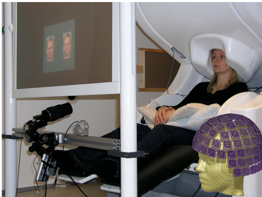
FIG. 8. MEG recording with a helmet-shaped neuromagnetometer. An infrared camera for simultaneous eye tracking can be seen in front of the subject. The inset on the right shows the 306-channel sensor array, normally located within the device immersed in liquid helium. (Courtesy of Veikko Jousmäki and Mika Seppä, Brain Research Unit, Helsinki University of Technology.)
